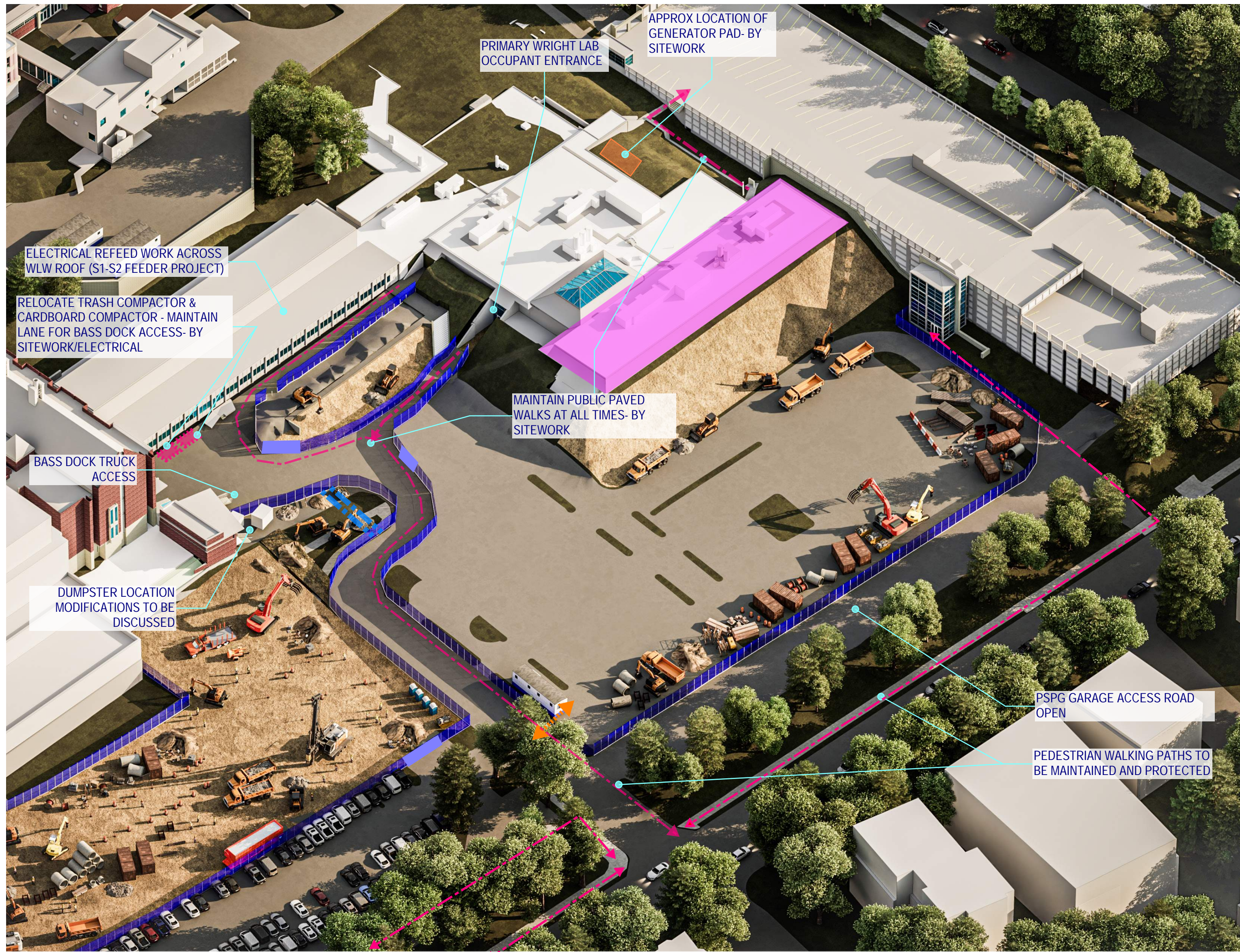
Yale PSEB - Wright Lab Additions and Renovations Logistics and Phasing Plan - Phase 1 - Site Mobilization and Enabling
