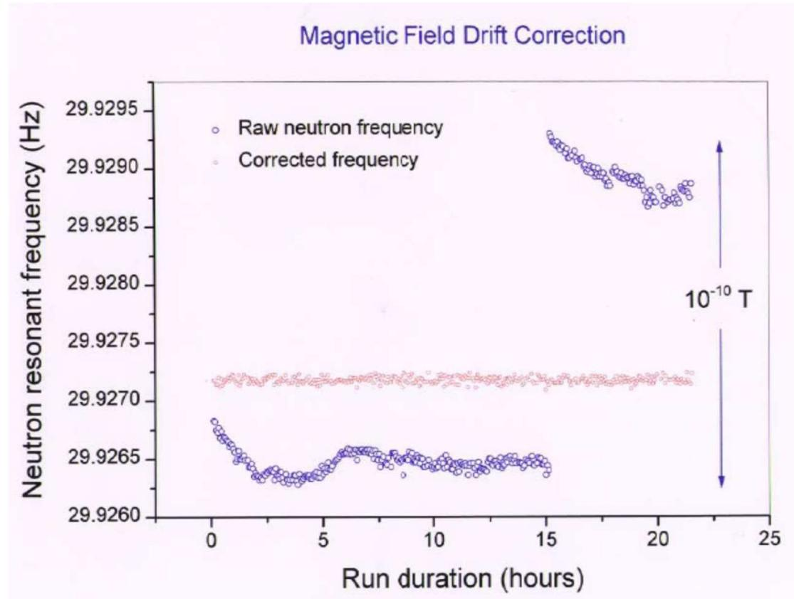
Data: ILL nEDM experiment with  $^{199}\text{Hg}$  co-magnetometer
