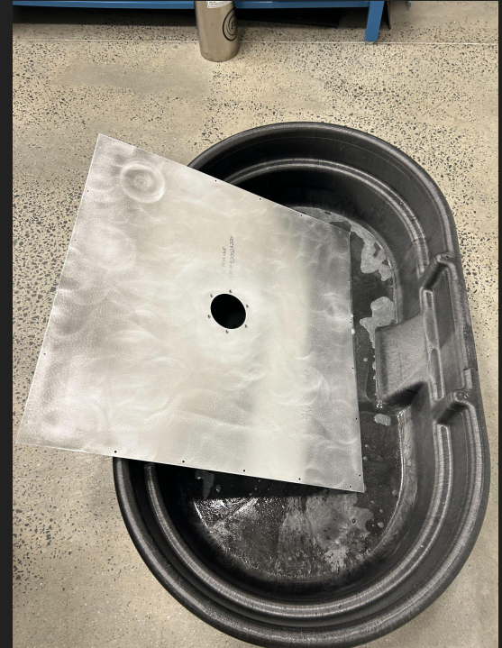
Cleaned with water→Simple Green→ethanol
