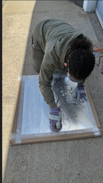
Orbital sanded, which produced aluminum dust
