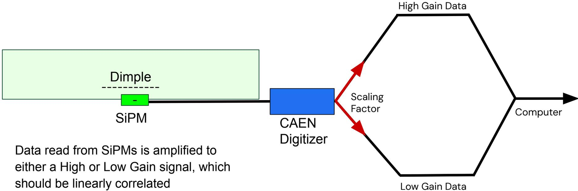
Data read from SiPMs is amplified to either a High or Low Gain signal, which should be linearly correlated
